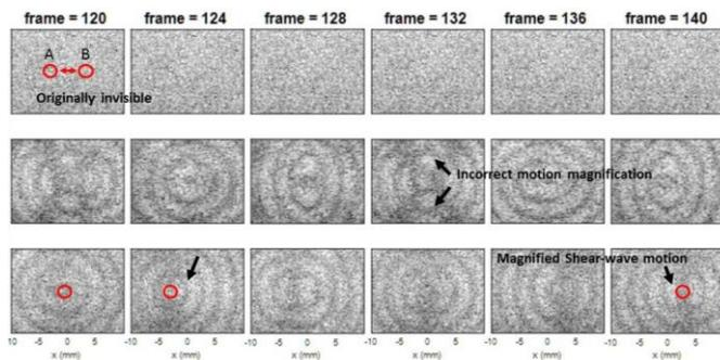
Fig. 3. Result of motion magnification. The first row is the original B-mode frames; the second row is the result with our previously proposed B-mode subwavelength vibration imaging; the third row is the result of our PCA-based motion magnification.
