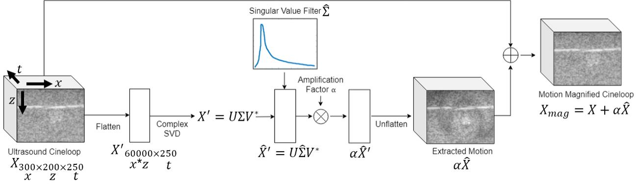
Fig. 1. Overview of the PCA-based motion magnification framework.
