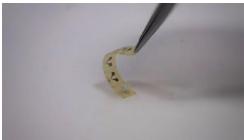
Fig. 5. Flexible strip of CMUT devices after peeling off from the silicon wafer.
