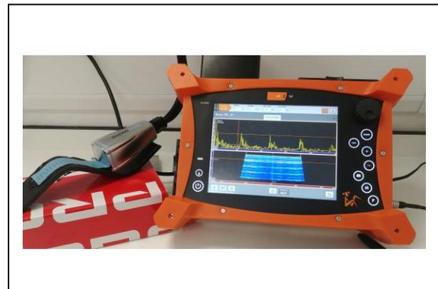
Fig. 3. Wall-thickness measurements achieved through curved sample with typical industrial testing apparatus.
