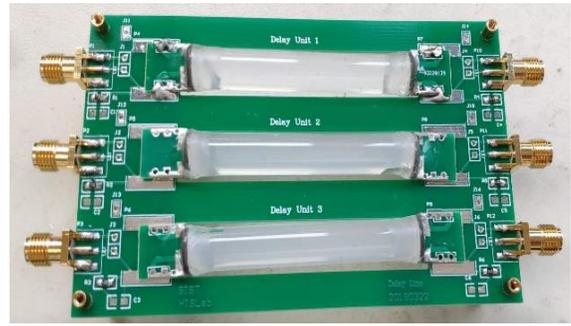
Fig. 3. The water made acoustic delay-line module
