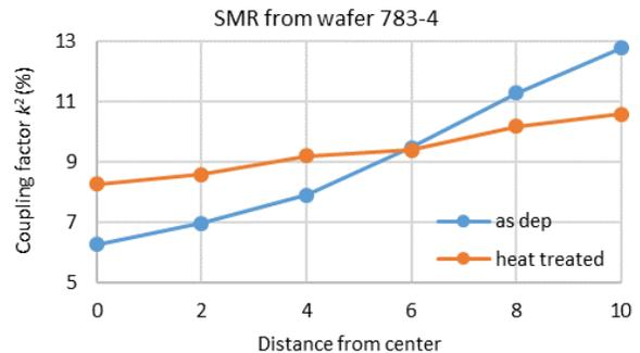
Fig. 5. Wafer radial variation of  $k^2$  in as deposited and heat treated samples.
