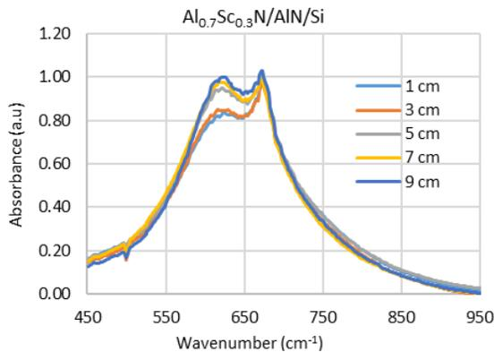
Fig. 3. FTIR spectra of five  $\text{Al}_{0.7}\text{Sc}_{0.3}\text{N}/\text{AlN}/\text{Si}$  samples distributed from the center to the edge of the Si wafers.
