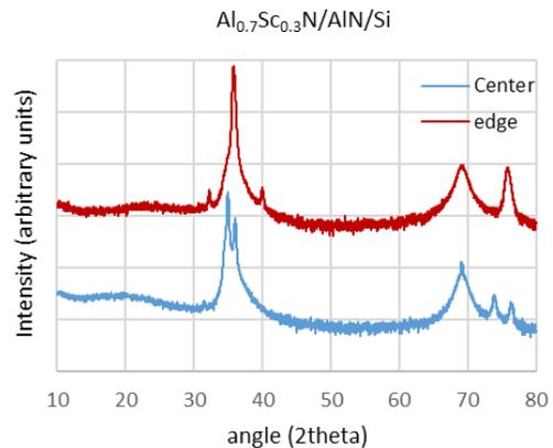
Fig. 1. XRD diffractogram of  $Al_{0.7}Sc_{0.3}N$  films at the center and at the edge of a 200-mm Si wafer. Note that the signal of the sample at the edge has been displaced for clarity.
