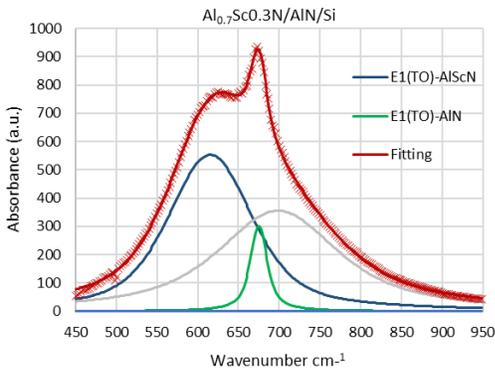
Fig. 2. FTIR spectrum of a representative  $\text{Al}_{0.7}\text{Sc}_{0.3}\text{N}/\text{AlN}/\text{Si}$  sample and the decomposition of the main features into E1(TO) peaks corresponding to the AlN seed layer (green) and to the AlScN layer.
