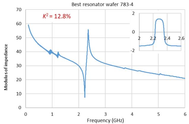
Fig. 4. Modulus of the impedance and phase of the best resonator measured at the edge of the wafer.
