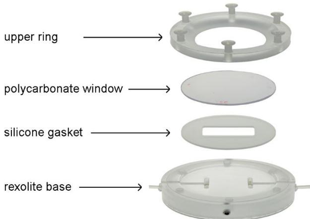
Fig. 1. Designed parallel-plate flow chamber (PPFC) [4].
