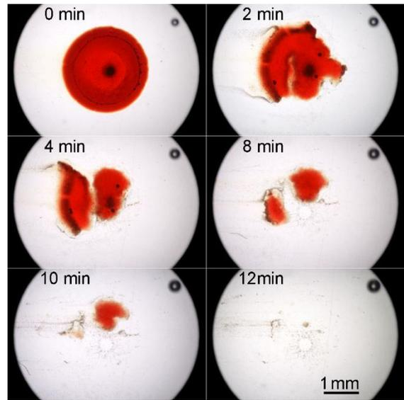
Fig. 5. Sequence of sonothrombolysis process taken every 2 min at 1 MHz.
