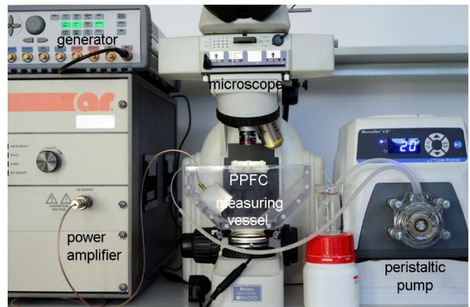
Fig. 3. Set-up for sonothrombolysis experiments.
