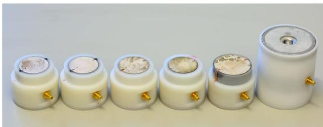
Fig. 2. Transducers designed for the experiment.
