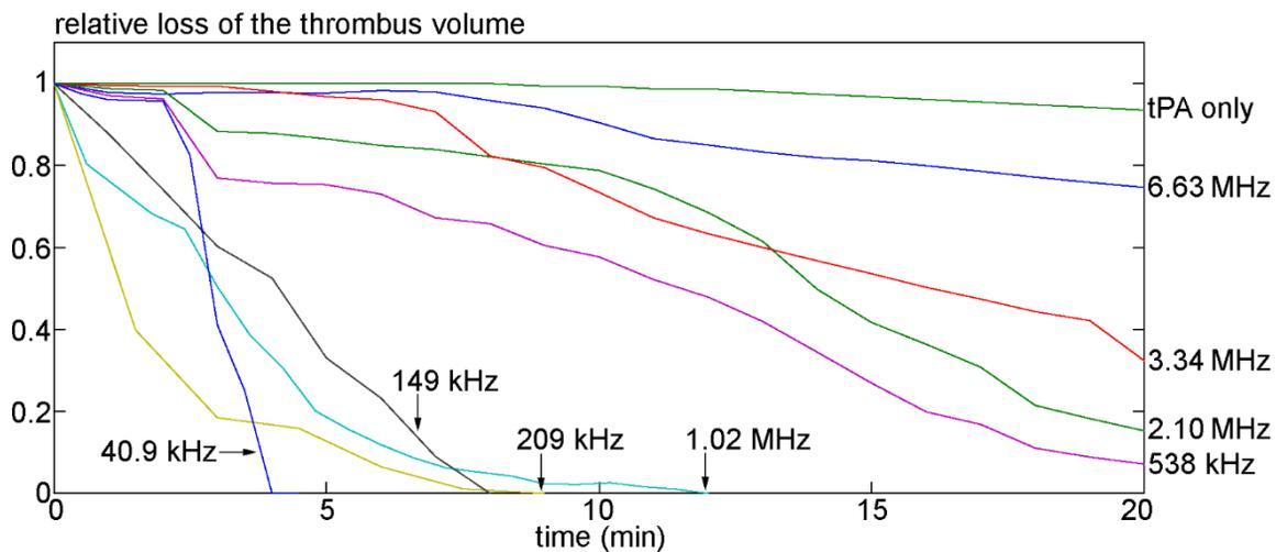
Fig. 4. Efficacy of the thrombus dissolution in the sonothrombolysis process at ultrasonic intensity  $I_{\text{SATA}} = 2\text{W}/\text{cm}^2$  and frequencies of 40.9 kHz - 6.63 MHz.
