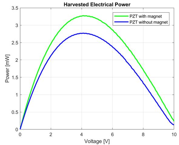
Fig. 5. The Measured harvested power by the PZT4 cube (blue) and the piezo-magnet stack (green) versus output voltage.
