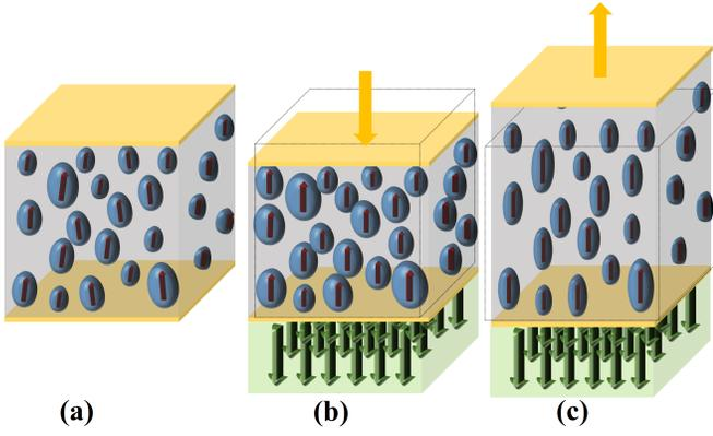
Fig. 1. PZT4 cube in (a) initial mode before ultrasonic stimulation. Piezo-magnet stack during ultrasonic powering in (b) compression, and (c) tension.
