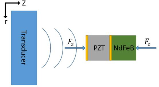
Fig. 2. Diagram of the piezo-magnet stack under the influence of mechanical force.
