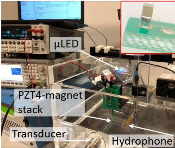
Fig. 4. Measurement setup with the piezo-magnet stack,  $\mu$ LED, ultrasonic transducer, and hydrophone. The inset shows enlarged piezo-magnet stack wirebonded to the PCB.
