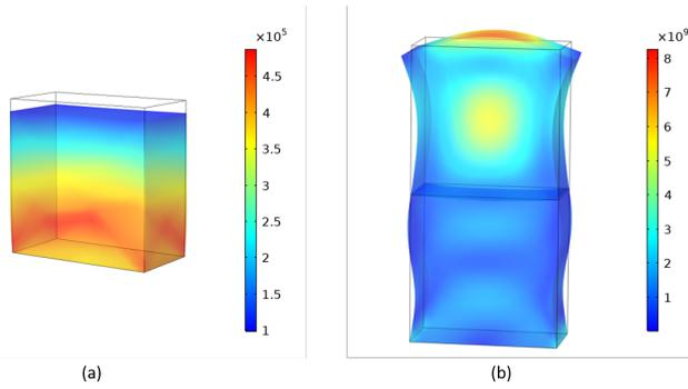
Fig. 3. Simulation of stress on PZT (a) and piezo-magnet stack (b) with a fixed boundary condition on the bottom and ultrasonic waves from the top.
