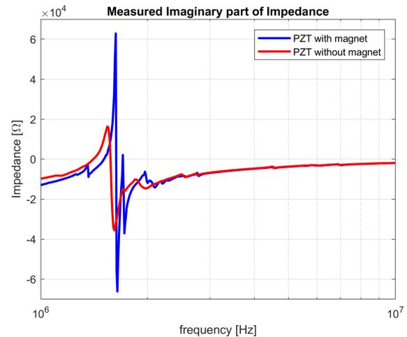
Fig. 6. Measured electrical impedance spectrum by network analyzer for PZT4 with (blue) and without (red) magnet.
