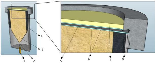
Fig. 2. Cross section view of transducer design (left) and detail of the connections (right)
