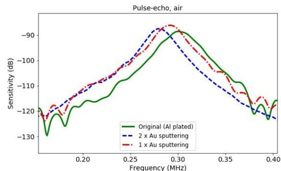
Fig. 6. Measured spectra of the pulse-echo response of the transducer in air. Original transducer and transducers with 1x 30 s sputtering of Au, and 2x 30 s sputtering of Au.
