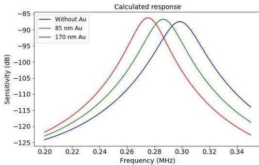
Fig. 7. Calculated spectra of the pulse-echo response of the transducer in air with different layers of Au deposited.
