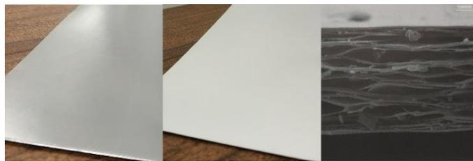
Fig. 1. Metalized side of ferroelectret (left), Non metalized side (centre), Cross-section SEM micrograph (right).
