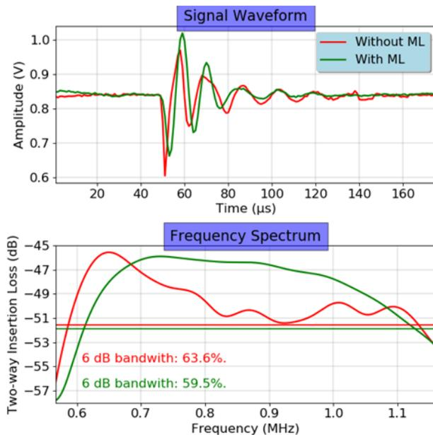
Fig. 8. Measured pulse-echo response in water immersion of transducers with and without matching layer. Up: impulse response. Bottom Spectra. The +40 dB Gain in the pulser receiver are not considered in the figure, so actual peak sensitivity is about -96 dB.
