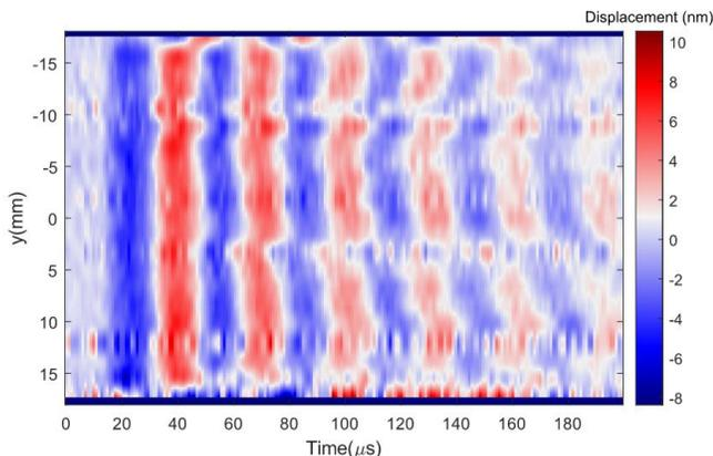
Fig. 5. Time evolution of the transducer surface displacement measured along one of the radiating surface diameters. Pulse excitation
