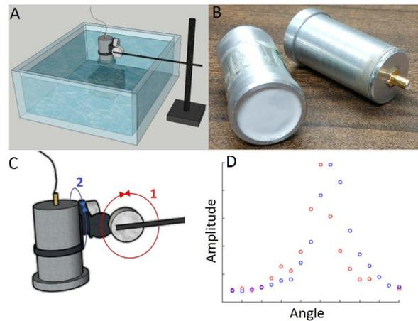
Fig. 3. Schematic representation of the experimental set-up for positioning the produced prototype transducer for water immersion pulse-echo characterization.
