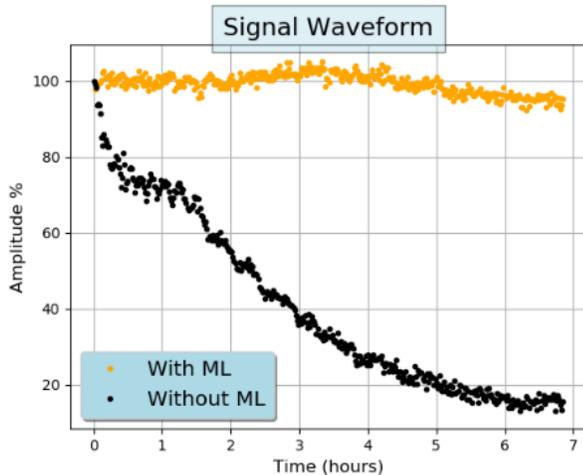
Fig. 4. Variation with time of immersion of the normalized echo amplitude for two prototype transducers: Transducer with unprotected Al metallization and transducer with one matching layer
