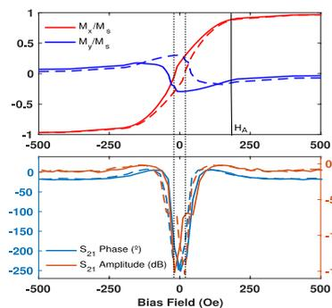
Figure 2:  $\text{TbCo}_2/\text{FeCo}$  thin film magnetization characteristics (top). Insertion Loss  $S_{21}$  (bottom)
