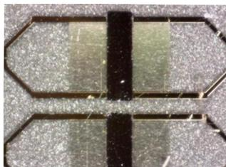
Figure 1: SAW delay line.
