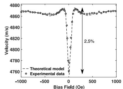
Figure 3: Theoretical calculation (dash) and experimental results (circles) for SH wave's velocity.
