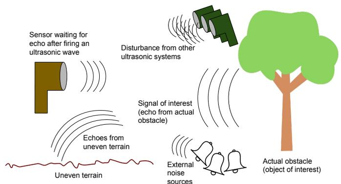
Fig. 1. Ultrasonic based system detecting an echo from an actual obstacle (tree) and being influenced by external disturbance sources such as noise in ultrasonic frequency range, other ultrasonic based systems and echoes from ground reflection
