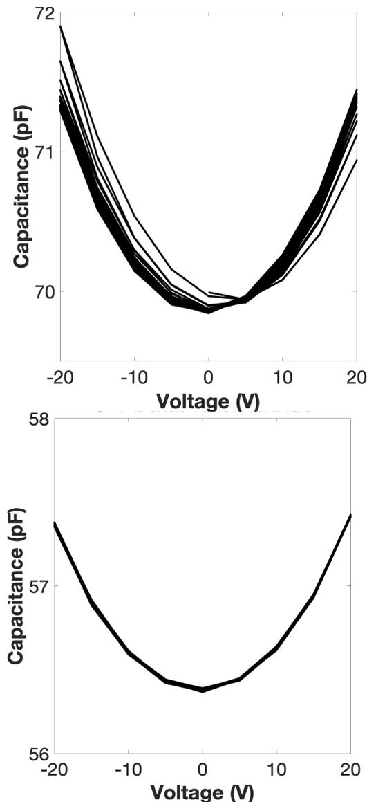
Figure 5: Capacitance vs. voltage (C-V) measurements of control device (top) and improved device (bottom)
