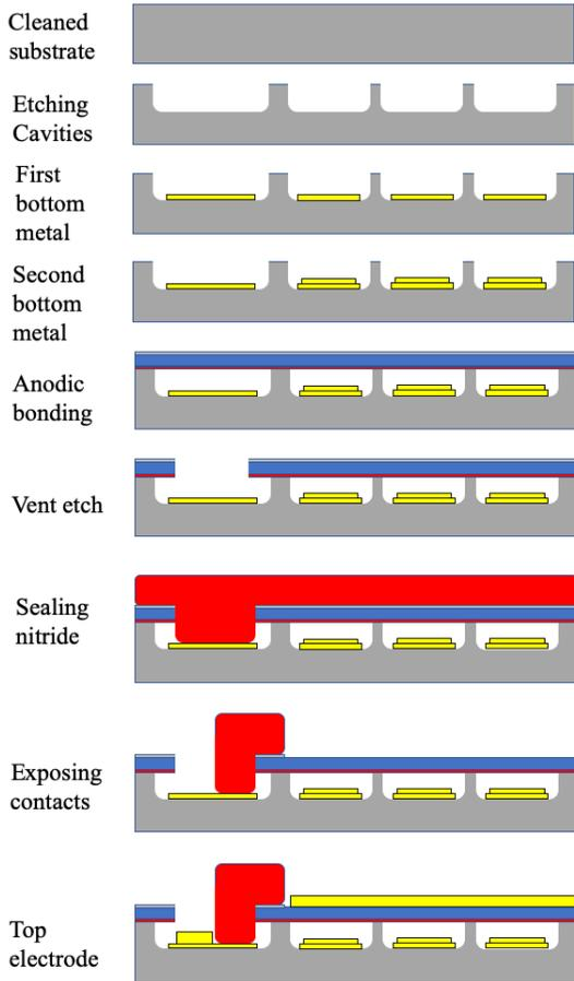
Figure 2: Process flow for fabrication of CMUTs
