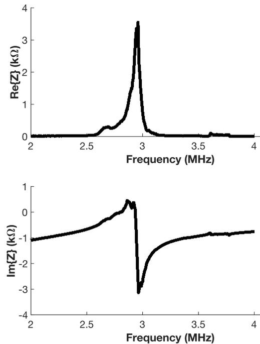
Figure 4: Real and imaginary parts of CMUT impedance
