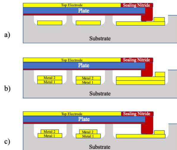
Figure 1: Cross sections of a) Conventional CMUT fabricated using anodic bonding process, b) Control device with the same gap height as a) with 2 metal steps, and c) the proposed device. For this run b) and c) were fabricated
