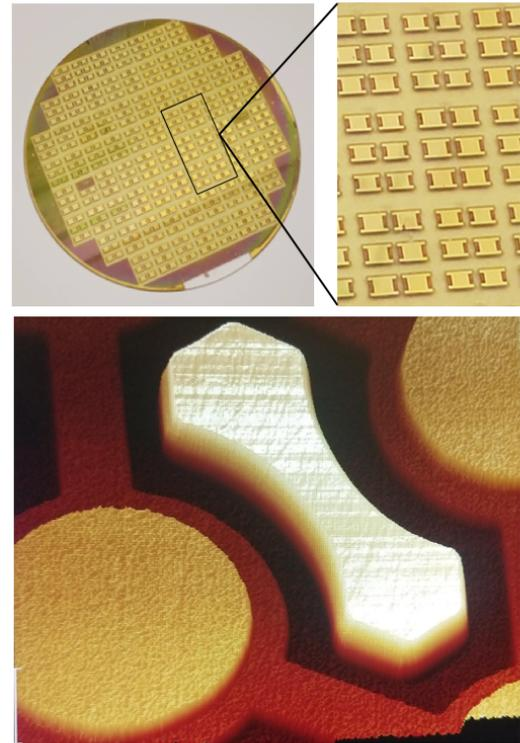
Figure 3: Photographs of the completed wafer with an AFM image showing the electrodes and post before bonding
