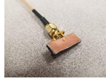
Figure 9: 4.3 GHz SAW temperature sensor packaged.
