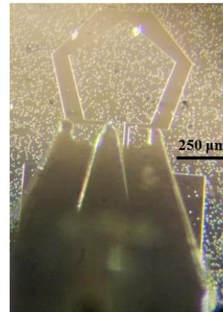
Fig. 5. Optical microscope image of the probed SMR during the 400°C test. The image shows the effect of the high temperature on the Ir-Au top electrode.
