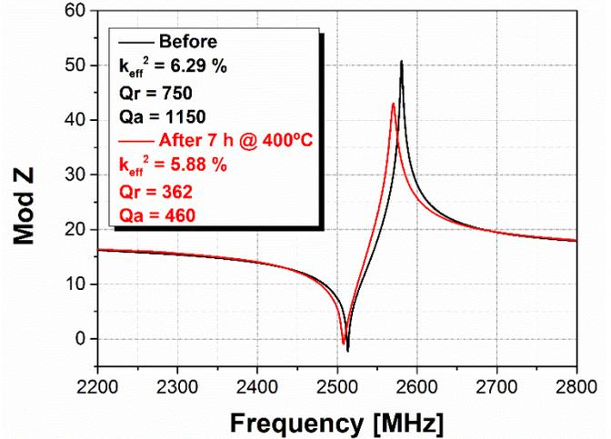
Fig. 4. Electrical impedance of the same SMR before and after the high temperature impact described in Fig. 3.
