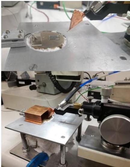
Fig. 2. RF probe station modified for high temperature operation. A Cu cap is used to prevent temperature dissipation (bottom picture).
