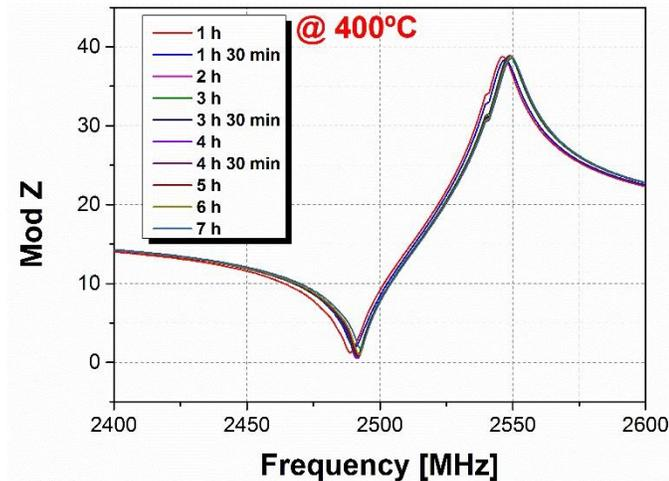
Fig. 3. Electrical impedances of an AlN-based SMR heated up to 400°C and maintained for seven hours.
