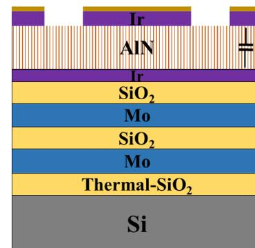
Fig. 1. Structure of the AlN-based SMR.
