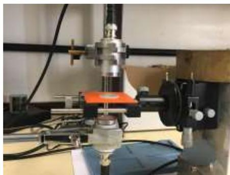
Fig. 1. Experimental setup employed for the ultrasonic air-coupled measurements (located in the “Instituto de Acustica CSIC”, Madrid, Spain).
