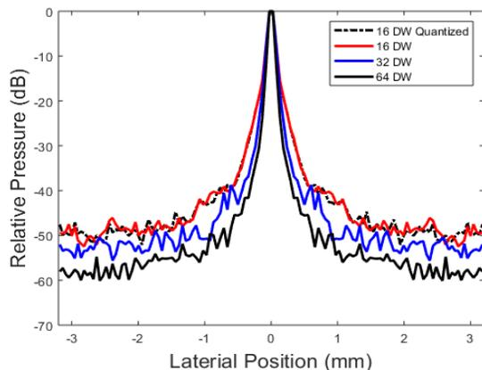
Fig. 2. The point spread function for 16, 32, and 64 diverging waves with the point source 6 mm away from the transducer face,  $\sim 0.15$  mm 6dB beam width
