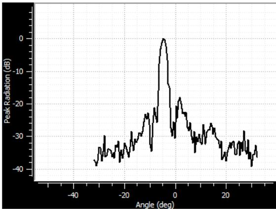
Fig. 4. The point spread function when measuring a wire target at 6mm depth, ~0.7 mm 6dB beam width
