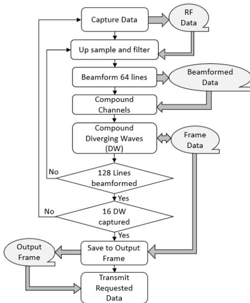
Fig. 3. The control flow implemented on the receive daughter cards
