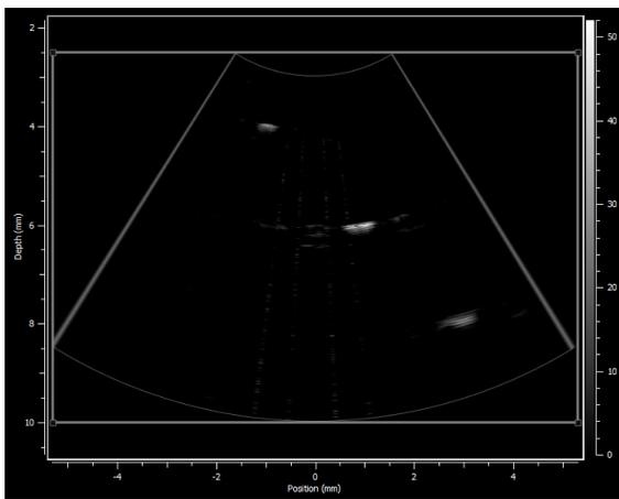
Fig. 5. Measurement of a wire phantom with 3 wire targets spaced apart displayed with 50 dB of dynamic range.
