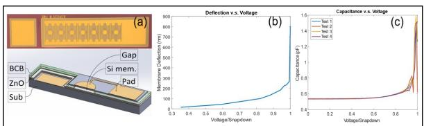
Fig.1 (a) Fabricated array and cross-sectional view of the ZnO CMUT devices (b) Deflection versus voltage changes measured by an optical profilometer. (c) Capacitive versus voltage changes measured with a Semiconductor Characterization System.
