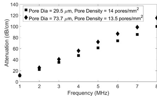
Figure 2: Frequency-dependent attenuation for two different porosities.
