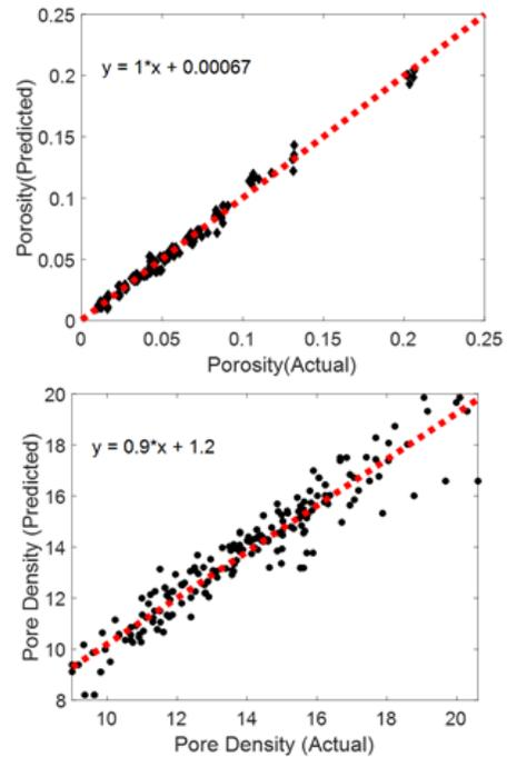
Figure 5 (Top) true porosity vs porosity predicted by neural network with 1x4 feature vector. (Bottom) true pore density vs pore density as predicted by neural network with 1x4 feature vector.
