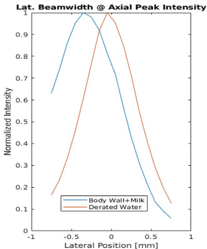
Fig. 3. The lateral beamwidth plot for the two waveforms measured through a sample abdominal wall+milk (blue) and the standard water (red) propagation path. The beamwidth plot is a function of the normalized pulse intensity integral.
