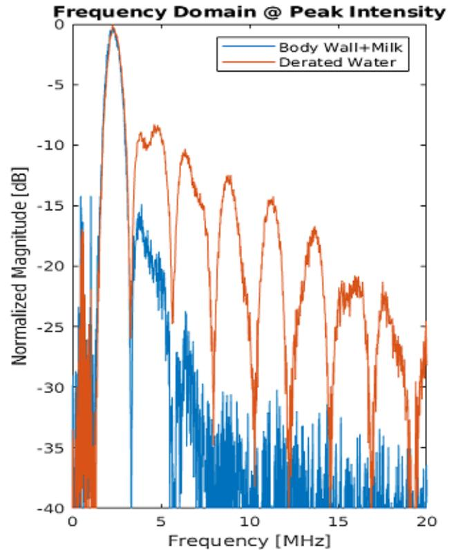
Fig. 2. The corresponding frequency domain plot for the two waveforms measured through a sample abdominal wall+milk (blue) and the standard water (red) propagation path. The y-axis is normalized by the peak magnitude of each waveform on a dB scale.
