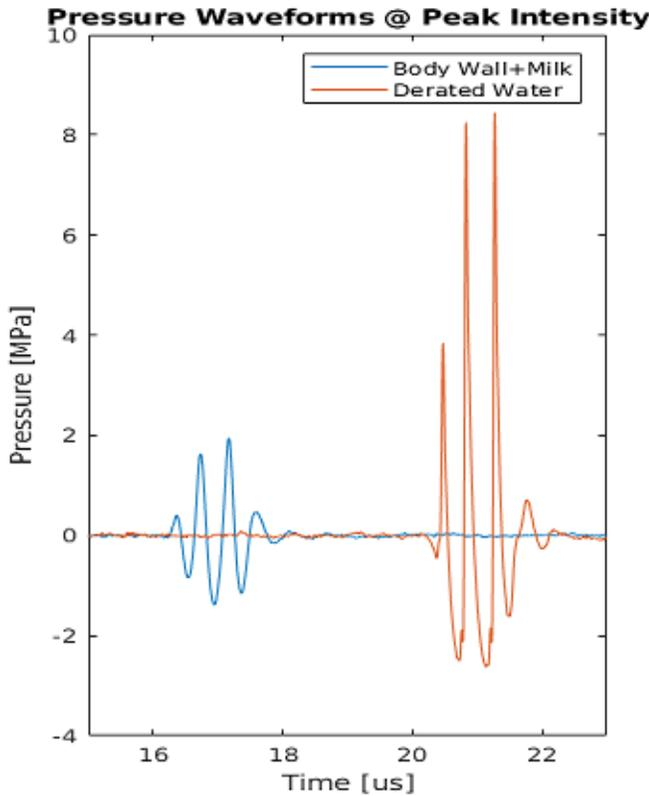
Fig. 1. The pressure waveforms at peak pulse intensity integral in space were plotted for both a sample abdominal wall+milk (blue) and the standard water (red) propagation path. For the waveform measured in water, a linear derating of 0.3 dB/MHz/cm is applied per MI metric definition.
