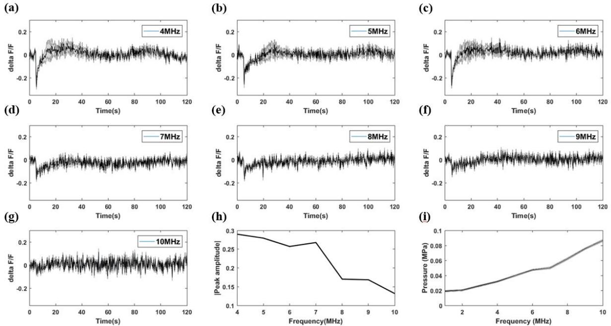
Fig 2.(a)-(g) Fluorescence intensity change frequency range from 10MHz to 4MHz. (F=Fluorescence intensity). (h) Absolute value of peak amplitude after stimulation. (i) Transducer output negative pressure. (Input electrical amplitude =  $90V_{PP}$ )
