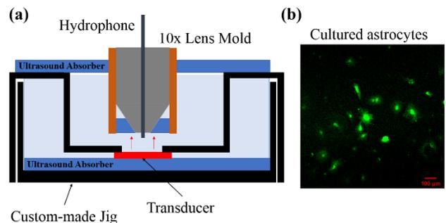
Fig 1.(a) Output measurement setup. (b) Calcium image of cultured astrocytes
