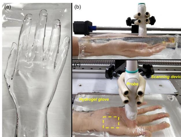
Fig. 1. A hydrogel glove and scanning device
