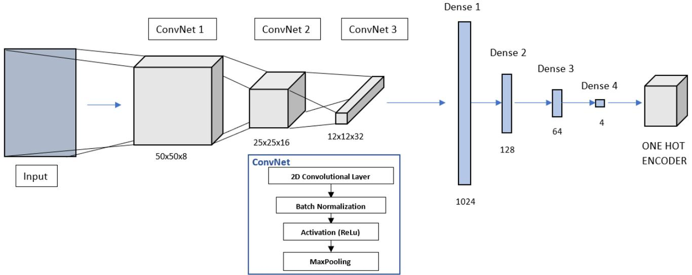
Fig. 3. VHC-CNN architecture.
