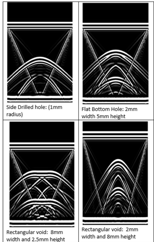
Fig. 2. B-Scan images for different flaw classes.
