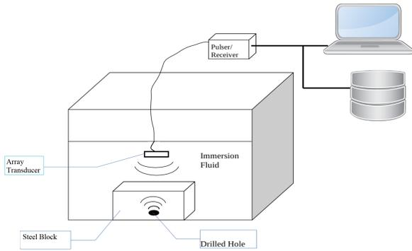
Fig. 1. Immersion setup with SDH using OnScale tools.
