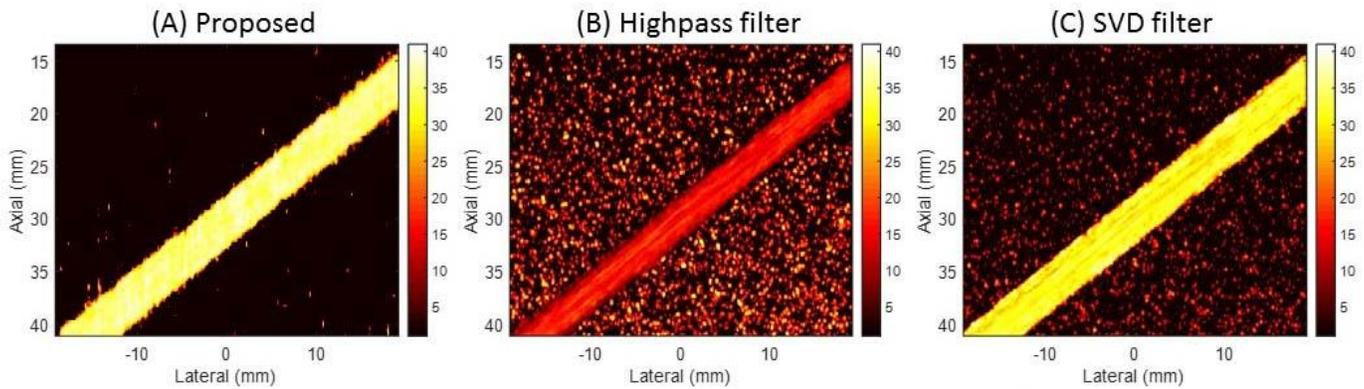
**Fig. 2** Power Doppler images of the simulated flow phantom with tissue clutter with the proposed convolutional encoder filtering (A), with the IIR high pass filtering (B), and with SVD filtering (C)
