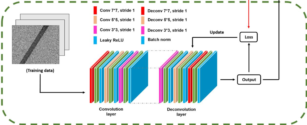
**Fig. 1** Schematic illustration of the simulation procedure and the autoencoder architecture. The data simulation is on the top left. Detailed procedure of the network is depicted on the bottom and power Doppler imaging is shown on the top right.
