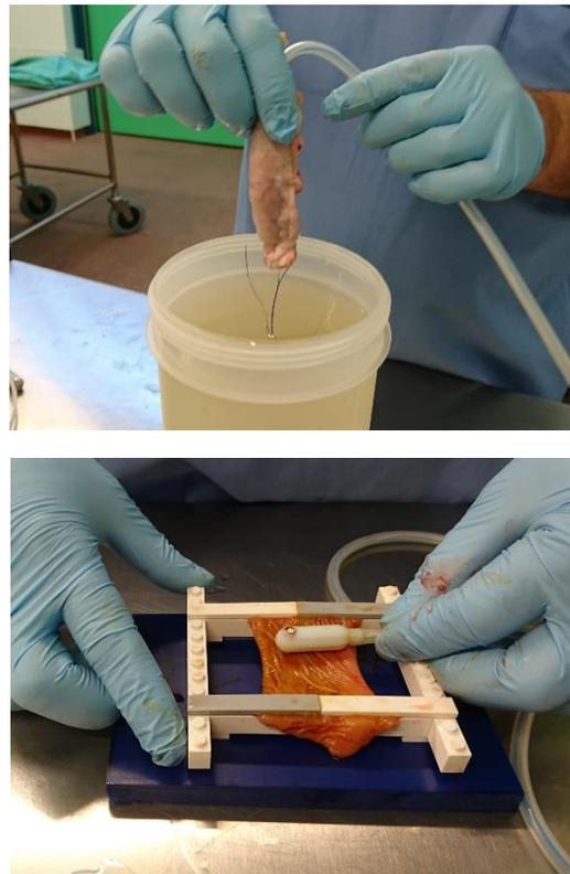
Fig. 4. *Ex vivo* scans (top) small bowel sample in air, (bottom) flattened small bowel sample in a gig in air.
