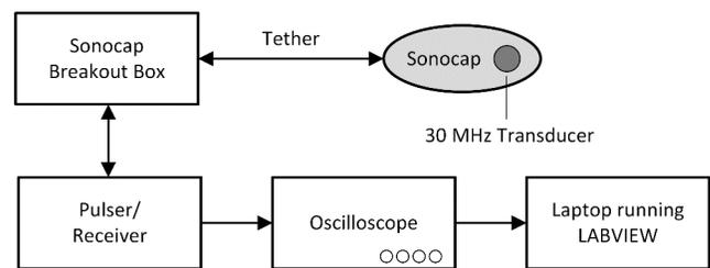
Fig. 3. Sonocap data-acquisition setup.
