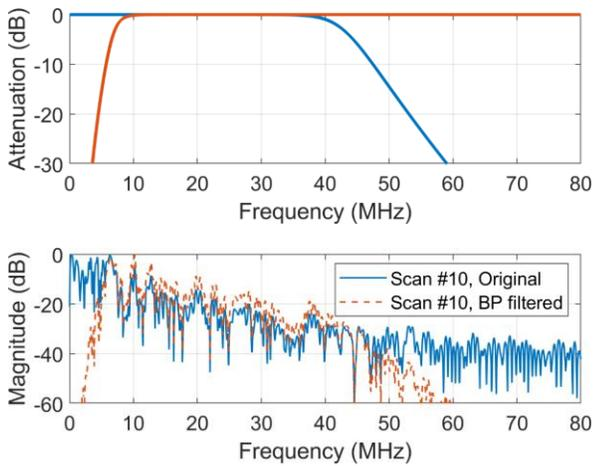
Fig. 5. Bandpass (BP) filtering: (top) low-pass (blue) and high-pass (orange) filter in the frequency domain, (bottom) example of a power spectrum of single A-Scan (Pig2, oesophagus, *in vivo* pullback), before and after filtering. A-Scan #10 before interpolation.
