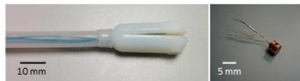
Fig. 1. Left: Sonocap before sealing. Right: Sonocap transducer.
