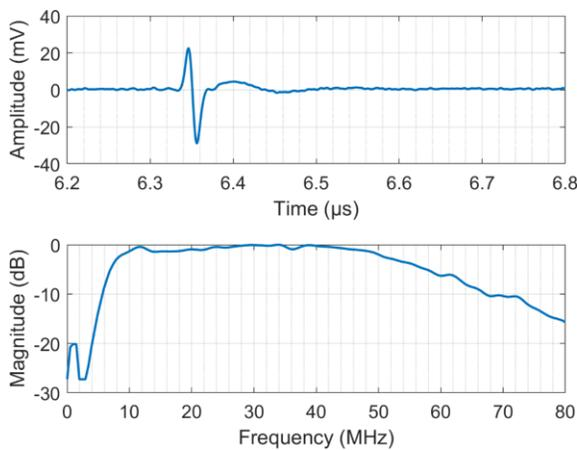
Fig. 2. Pulse-echo response and frequency spectrum of the single element transducer. Measured on a glass reflector, with a gain of 20 dB and 256 averages.
