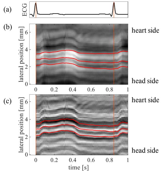
Fig. 2. (a) ECG. (b) Estimated displacements by the block matching method for the envelope of RF signals. (c) Estimated displacements by the block matching method for the difference signals of the envelope of RF signals between neighboring beams in the longitudinal direction. Change of maximum amplitudes of echo envelope and that of subtracted image in the longitudinal direction are shown in (b) and (c), respectively.
