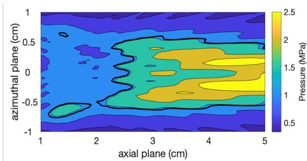
Fig. 1: Measured PW Doppler field of the Philips S5-1 in water. The black contour shows the 6 dB down from the maximum region.
