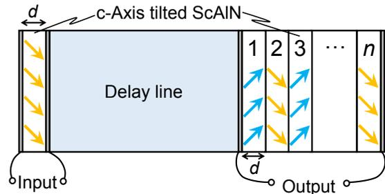
Fig. 1. BAW transformers based on c-axis zig-zag ScAlN stack.
