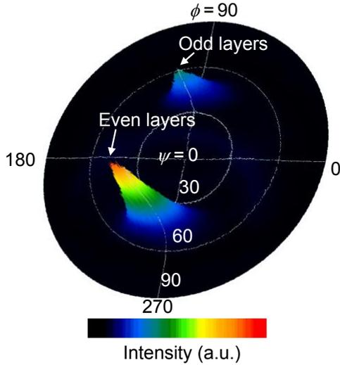
Fig. 3. (0002) pole figure of 4-layers ScAlN film stack.
