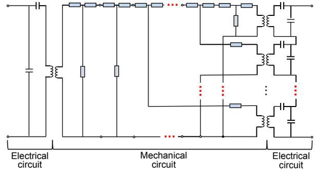
Fig. 5. Mason's equivalent circuit model based on polarity inverted.
