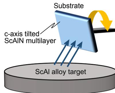
Fig. 2. Deposition method of c-axis zig-zag ScAlN multilayers.
