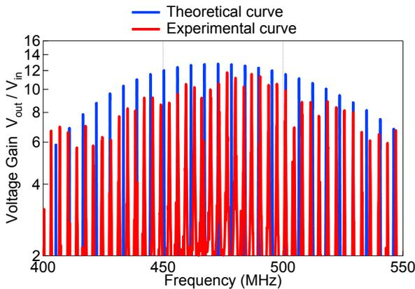
Fig. 4. Voltage gain of the 4 layers BAW transformer.
