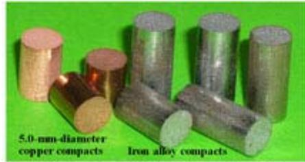
Fig. 2 5-mm-diameter copper and iron alloy powder compacts using 20 kHz ultrasonic compacting equipment with upper and lower vibration punches.
