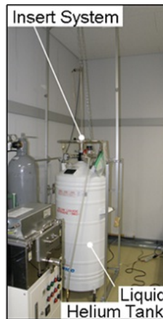
(b) Cryogenic evaluation system
