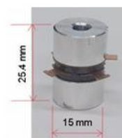
Fig. 3 Picture of the proposed Langevin transducer.
