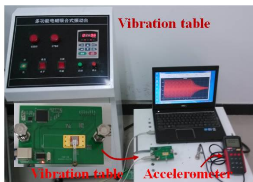
Figure 1 the developed SAW accelerometer and measurement setup
