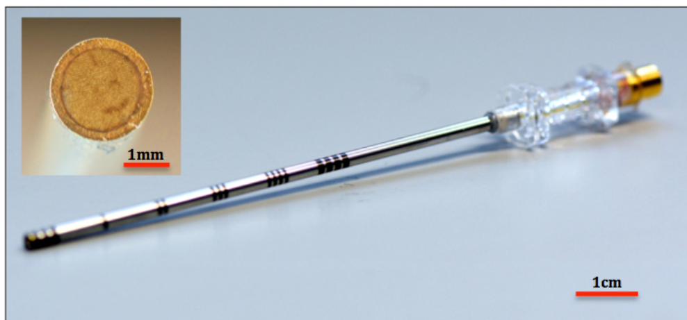
Finished forward facing single element ultrasound transducer in a needle.
