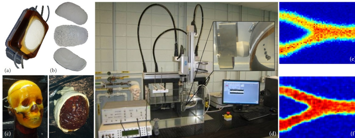
Fig.1. (a) Custom made phantom used in our previous work; (b) Structure of the skull in these phantoms (top to bottom: outer, middle, and inner layers, respectively); (c) Additionally, a more realistic phantom has been used in this paper (left: perspective view; right: inner view with the brain and vessels); (d) Scanner and the experiment setup; (e) The best result obtained using our previous work; (f) Proposed method.
