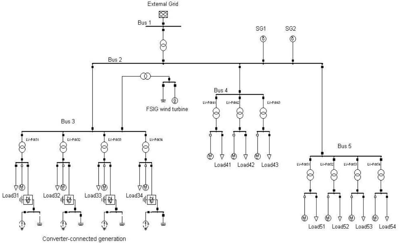
Fig.2. Single line diagram of the test network
