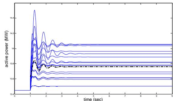
Fig. 8. Model response with averaged parameters (thick dashed line) and responses with individual sets of parameters
