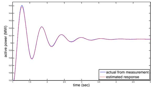
Fig. 6. Response following 10% reduction in torque of SG1
