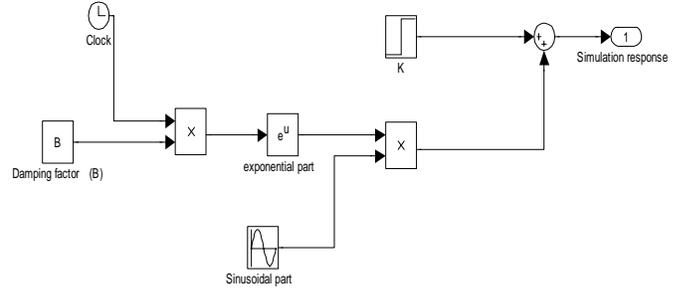
Fig. 1. MATLAB/Simulink representation of equation (3)
