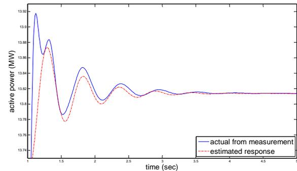
Fig. 7. Response following 25% reduction in torque of SG2
