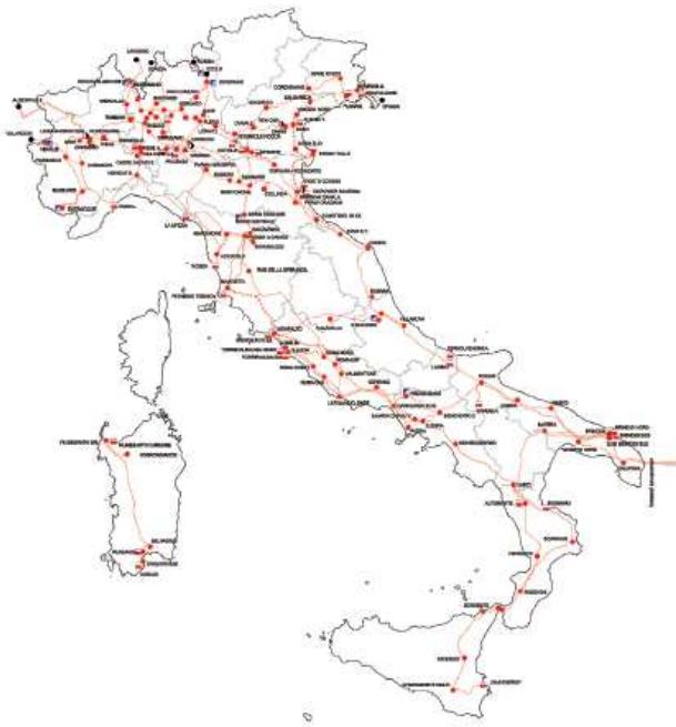
Fig. 11. Overview of the Italian 400 kV transmission grid
