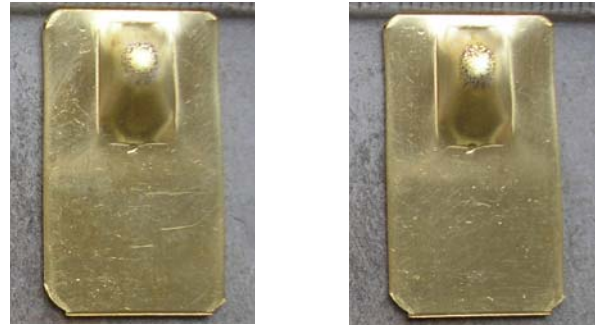
Fig. 3. Standard etchings - Smallest and largest areas on gap electrodes of Manufacturer I surge arresters
