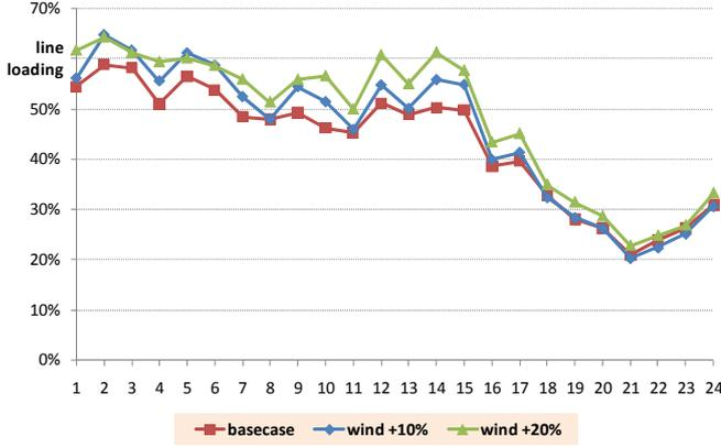
Fig. 6. Loading of the lines connecting nodes 6 and 8.
