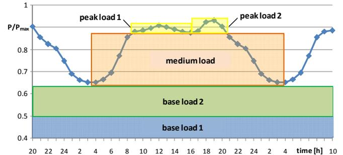
Fig. 2. Segmentation of the load curve.
