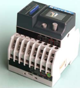
Figure 4. Prototype of the three-phase, voltage-and-current, 61000-4-30 Class A power quality monitor. The digital camera influence can be seen in the SD memory card, which holds up to 2 000 MB of data. Standard DIN-rail mounting means installation is cheap and quick.
