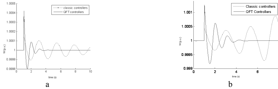
Fig. 22. Dynamic responses for \omega with considering transitory 3-phase fault at the infinite bus for heavy load (operating point 4)
