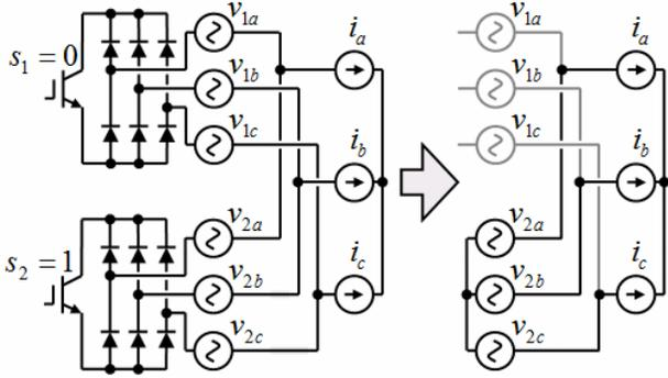
Fig. 8. Equivalent circuit when  $S_1$  is *off* and  $S_2$  is *on*
