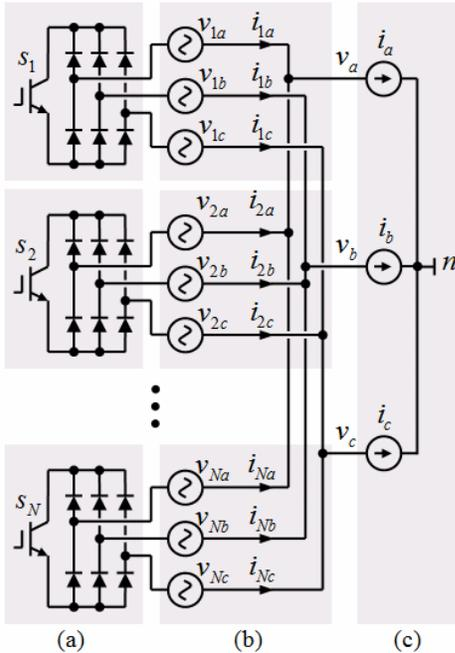
Fig. 4.  $N \times 1$  VeSC (a) three phase switches (b) voltage inputs (c) output
