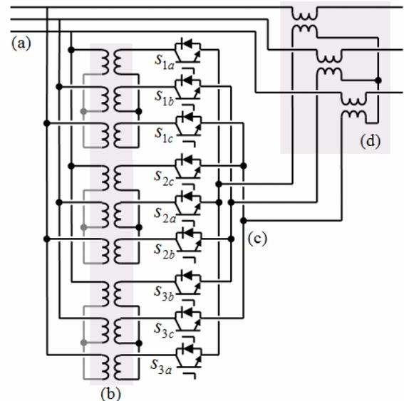
Fig. 18. VeSC based UPFC (a) transmission line (b) phase shift transformers (c)  $3 \times 1$  three-phase VeSC (d) series injection transformer.
