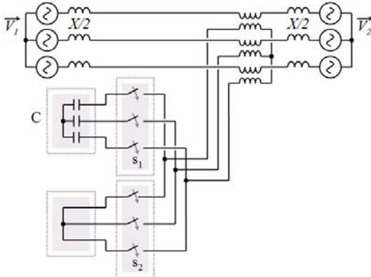
Fig. 11. Vector switching converter representation of the  $\Xi$  controller
