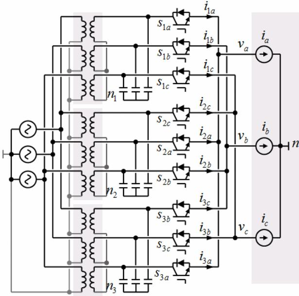
Fig. 3. Additional details about the implementation for the converter in Fig. 1. Capacitors decouple the transformer's leak inductance to behave as a voltage source.
