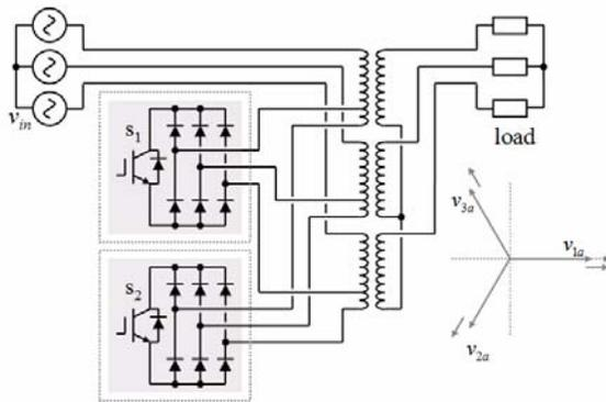
Fig. 20. Two driven switches tap changer, one driven switch is used for each tap. A secondary tap configuration can be derived in the same way.
