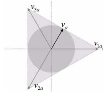
Fig. 2. Attainable output voltage for three input voltage with  $120^\circ$  phase shift
