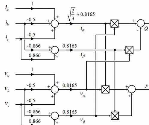
Fig. 14. Power Meter block by the static reference frame
