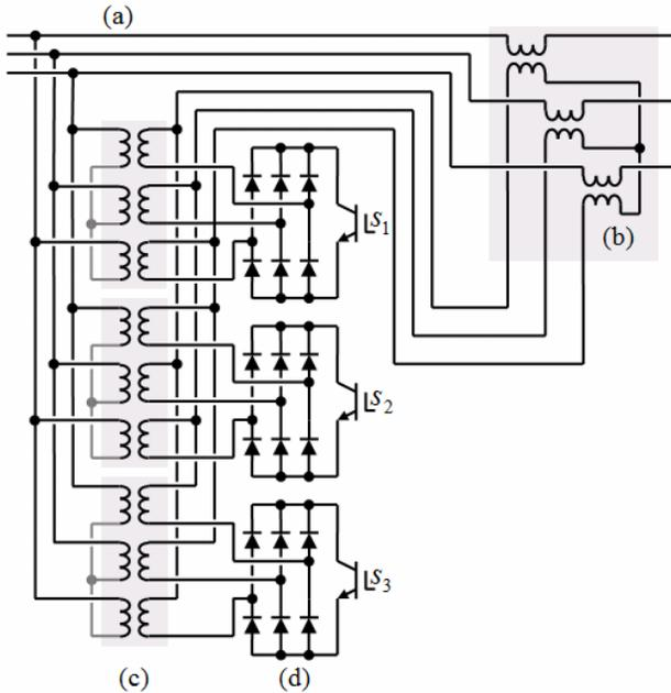
Fig. 19. SVEsC based UPFC (a) transmission line (b) series injection transformer (c) phase shift transformers (d) 3x1 three-phase SVEsC.
