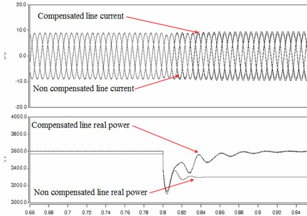
Fig. 15. Current and active power for the compensated and non-compensated system under a disturbance
