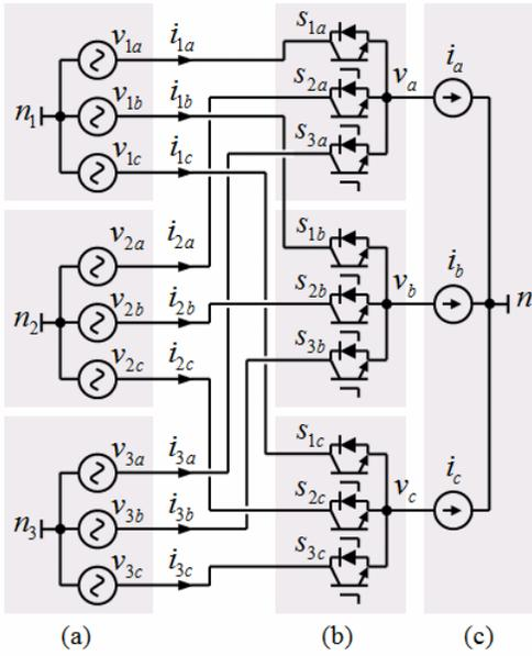
Fig. 1. Three-phase  $3 \times 1$  vector switching converter
