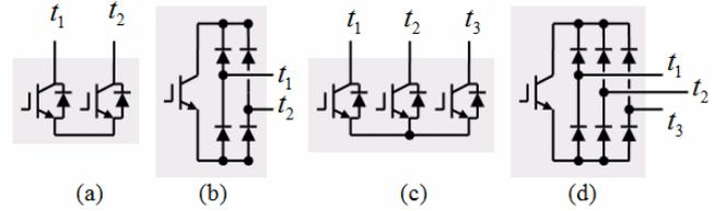
Fig. 6. (a) and (b) two-ports bidirectional switches (c) and (d) three-ports bidirectional switches
