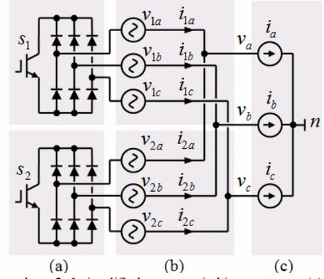
Fig. 5. Three-phase  $2 \times 1$  simplified vector switching converter (a) three-phase switches (b) three-phase input voltages (c) three-phase output
