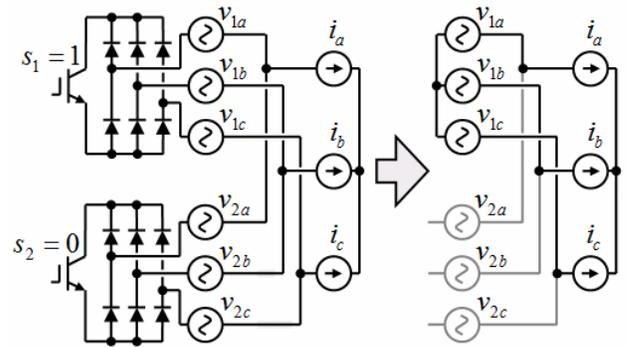
Fig. 7. Equivalent circuit when  $S_1$  is on and  $S_2$  is off.
