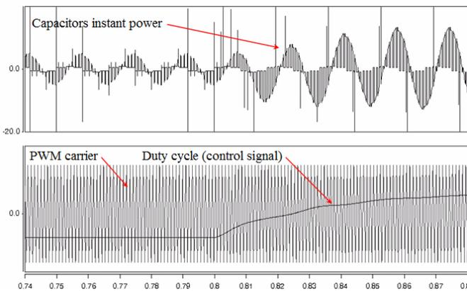
Fig. 16. Capacitors' instant power and duty cycle with the PWM carrier during the disturbance
