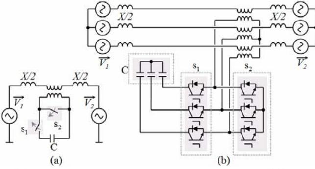
Fig. 9.  $\Xi$  controller (a) single phase circuit (b) three-phase circuit [16]
