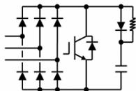
Fig. 17. One snubber circuit is employed for each switch in the proposed simplified topologies.
