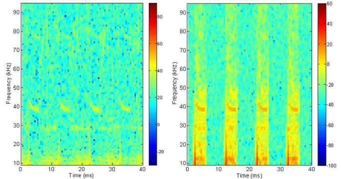
Fig. 4. Spectrogram of the voltage (left) and the current (right) when the lamp is supplied from the public grid.
