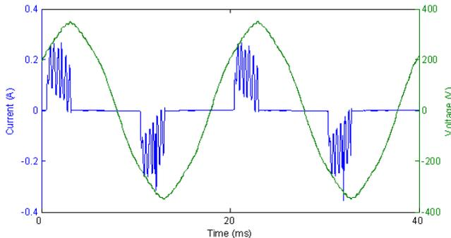
Fig. 2. Voltage (green) and current (blue) when a fluorescent lamp is supplied from a 100 kVA backup generator. The horizontal scale is from zero to 40 ms.
