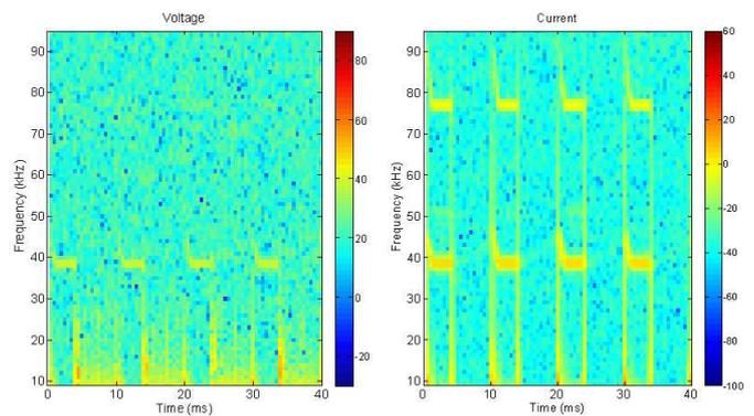
Fig. 6. Spectrogram of the voltage (left) and the current (right) when the lamp is supplied from a 37-kVA synchronous generator.
