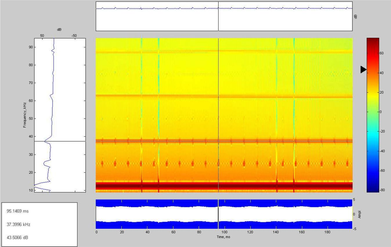
Fig. 9. Time-frequency representation of the current taken by an LCD screen while the PLC is transmitting.
