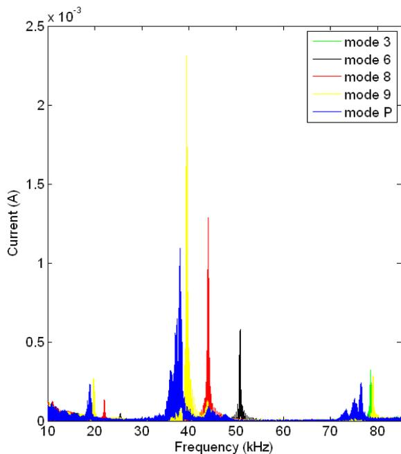
Fig. 7. Spectrum of the current taken by a compact fluorescent lamp close to an induction cooker. The different colors correspond to different states of the induction cooker. The horizontal scale is from 10 to 90 kHz.
