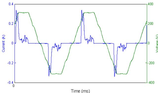
Fig. 3. Voltage (green) and current (blue) when a fluorescent lamp is supplied from a 37 kVA synchronous generator. The horizontal scale is from zero to 40 ms.
