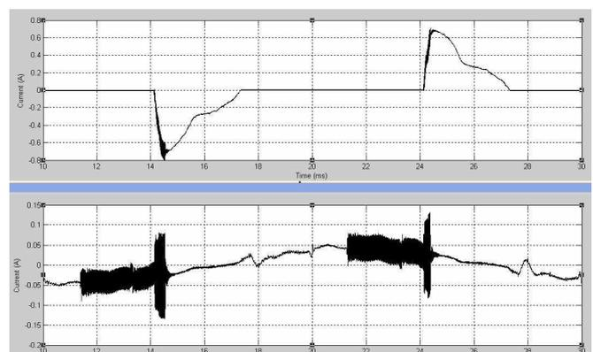
Fig. 8. Current drawn by a CFL 11 W (top) and by PLC disturbance source (bottom). The horizontal scale is from 10 to 30 ms.
