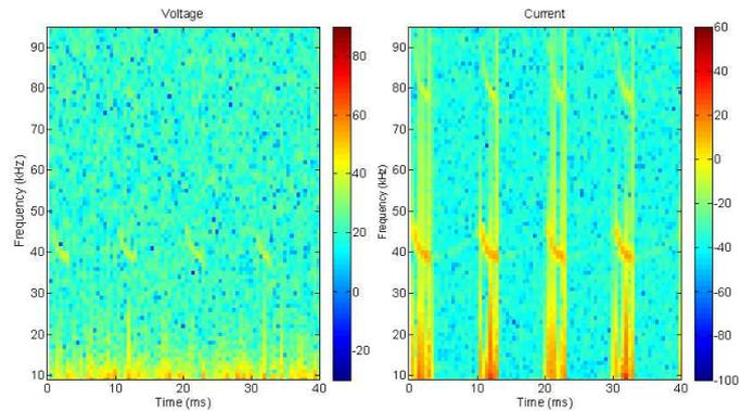
Fig. 5. Spectrogram of the voltage (left) and the current (right) when the lamp is supplied from the 100-kVA backup generator.
