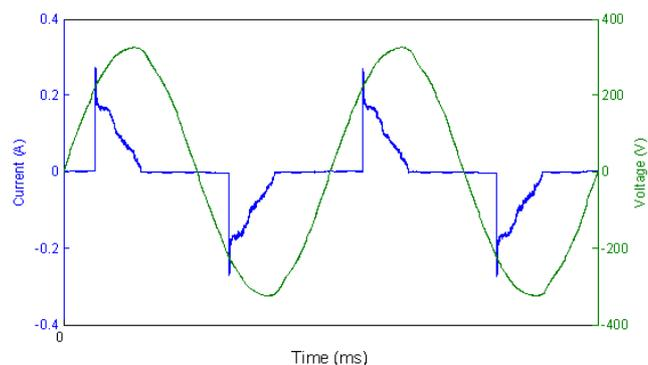
Fig. 1. Voltage (green) and current (blue) when a fluorescent lamp is supplied from the public grid. The horizontal scale is from zero to 40 ms.
