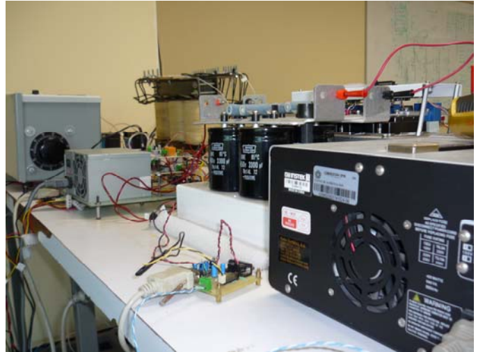
Fig. 5 VSC and transformers
