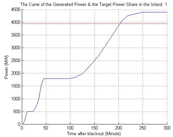
Figure V: Generation Capability in Island 1 for Receiving the 39.4112 p.u. Target Power
