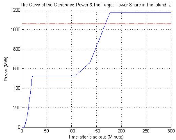
Figure VI: Generation Capability in Island 2 for Receiving the 10.5888 p.u. Target Power
