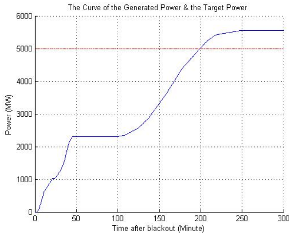
Figure IV: Generation Capability in Total System for Receiving the 50 p.u. Target Power
