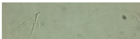
(a) RI of liquid does not equal RI of cellulose fiber.
