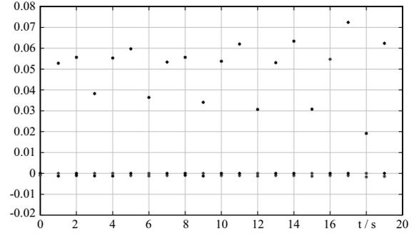
Fig. 8. Trend of eigenvalues, fault at line 02\_25 – unstable case
