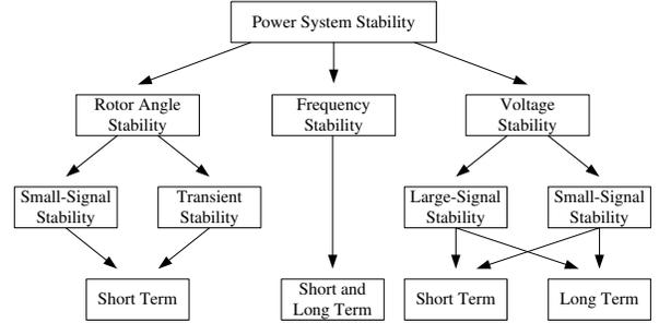
Fig. 4. Classification of power system stability [5]
