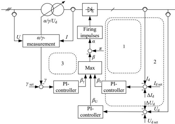
Fig. 10. HVDC control loops
