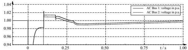
Fig. 12. AC-voltages during fault at inverter AC-side
