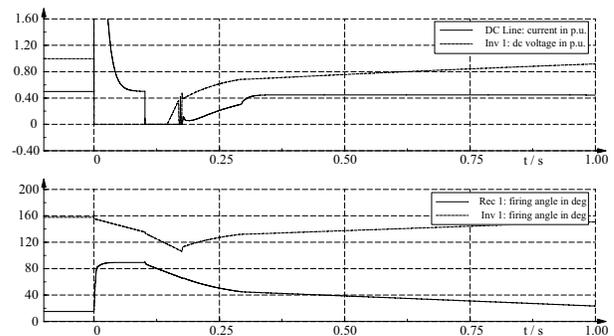
Fig. 13. DC-parameters and firing angles during fault at inverter AC-side
