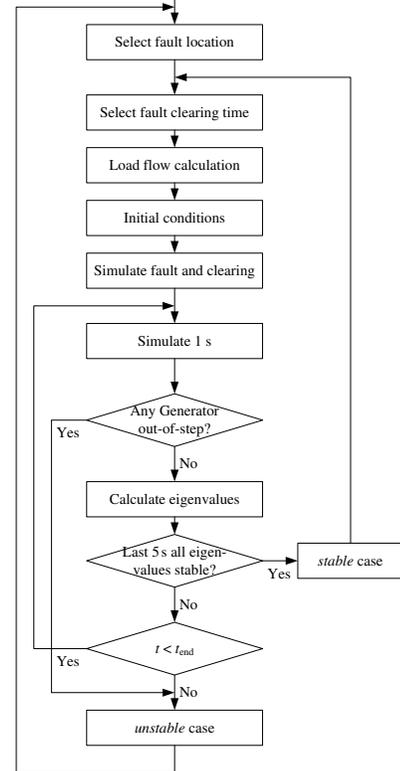
Fig. 9. Flow chart of proposed stability analysis method
