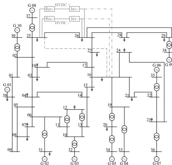
Fig. 1. Modified IEEE 10 Generator 39 Bus System
