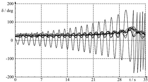
Fig. 7. Rotor angle oscillations, fault at line 02\_25
