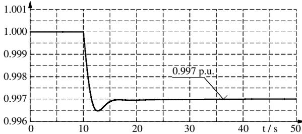
Fig. 2. Generator test: speed in p.u.
