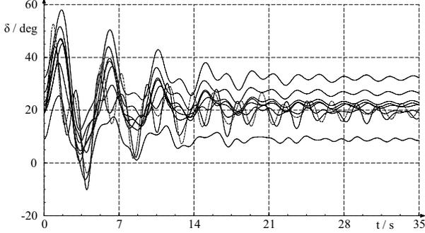
Fig. 5. Rotor angle oscillations, fault at bus 13
