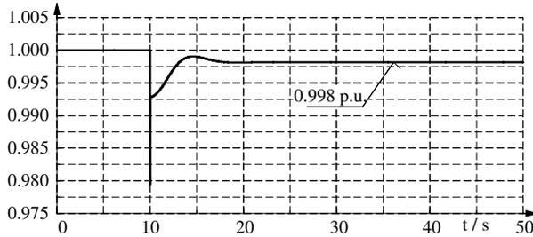
Fig. 3. Generator test: terminal voltage in p.u.
