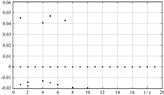
Fig. 6. Trend of eigenvalues, fault at bus 13 – stable case
