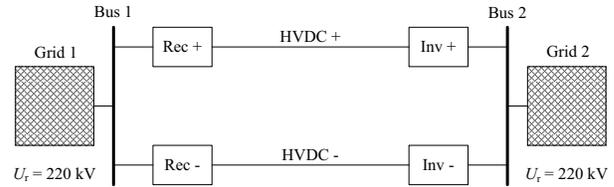
Fig. 11. Test of HVDC connection
