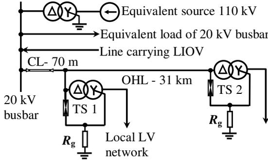
Fig. 1. Equivalent diagram of the studied network (used acronyms: CL – cable line; OHL – overhead line; LIOV- lightning induced overvoltage; TS – transformer substation).
