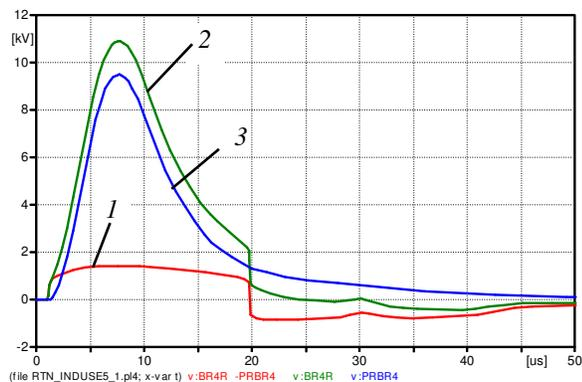
Fig. 9. The transient voltages at connection point of low voltage consumer supplied from TS1 between: 1 –phase-neutral; 2 – phase-reference earth; 3 - neutral-reference earth.
