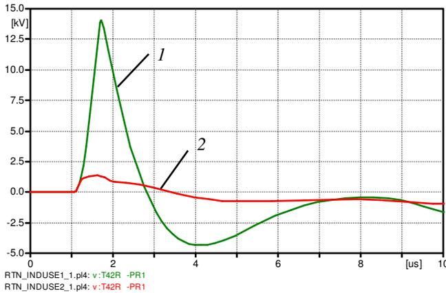
Fig. 4. Potential difference between low voltage terminal and neutral (connected to ground) at TS1: 1 - without low voltage surge arresters; 2 - with low voltage surge arresters.
