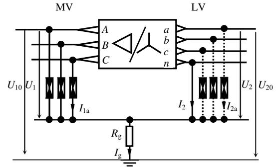
Fig. 3. The notations of main studied parameters at each transformer substations (MV- medium voltage terminals; LV-low voltage terminals;  $R_g$ - resistance of ground).
