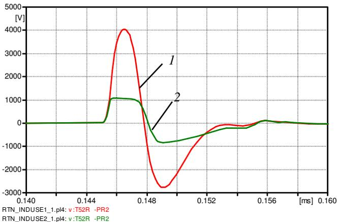
Fig. 5. Potential difference between low voltage terminal and ground at TS2: 1 - without low voltage surge arresters; 2 - with low voltage surge arresters.
