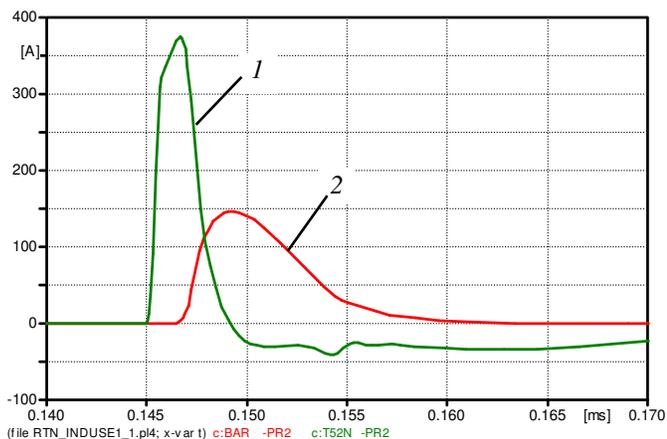
Fig. 6. The transient currents at TS2 through: 1 – medium voltage surge arrester; 2 – connection to ground of low voltage network neutral.
