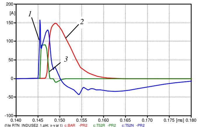
Fig. 7. The transient currents through TS2: 1 – connection to ground of low voltage network neutral; 2 – medium voltage surge arresters; 3 – low voltage surge arresters.
