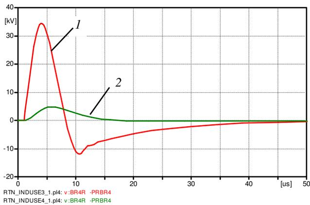
Fig. 8. The phase-neutral voltage at point of connection of low voltage consumer supplied by TS1: 1 – with no load connected; 2 – with a usual load of  $40 \Omega$ .
