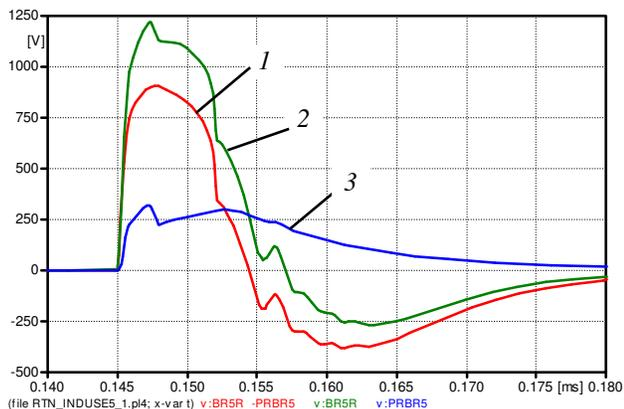
Fig. 10. The transient voltages at connection point of low voltage consumer supplied from TS2 between: 1 –phase-neutral; 2 – phase-reference earth; 3 - neutral-reference earth.
