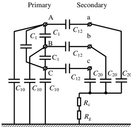
Fig. 2. The capacitances added to complete the saturable power transformer (250 kVA, 20/0.4 kV) model in ATP-EMTP ( $C_1 = 5$  nF;  $C_{10} = 0.5$  nF;  $C_{12} = 5$  nF;  $C_{20} = 10$  nF;  $R_c$  – the resistance of neutral connection to ground;  $R_g$  – the resistance of ground, 4  $\Omega$ ).
