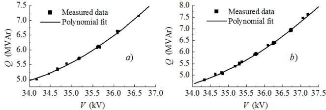
Fig. 2. Measured values and polynomial fit from the experiment of: voltage decrease a) and voltage increase b).
