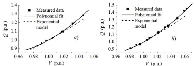
Fig. 4. Measured data normalized with  $V_n$  and  $Q_n$ , polynomial fit and exponential model for: voltage decrease a), and increase b).
