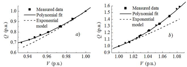
Fig. 3. Measured data normalized with  $V_0$  and  $Q_0$ , polynomial fit and exponential model for: voltage decrease a), and voltage increase b).
