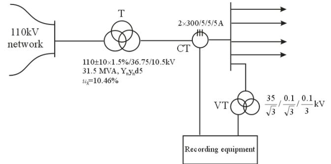
Fig. 1. Simplified experimental schema.
