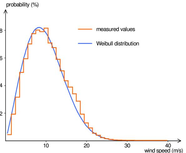
Fig. 2. Wind speed distribution at FINO measurement station.
