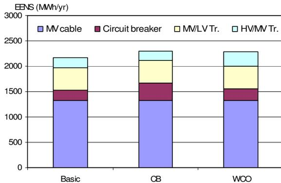
Fig. 9. The comparison of EENS for all three variants.
