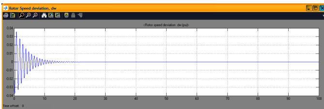
Fig. 13. Rotor speed deviation, d\omega
