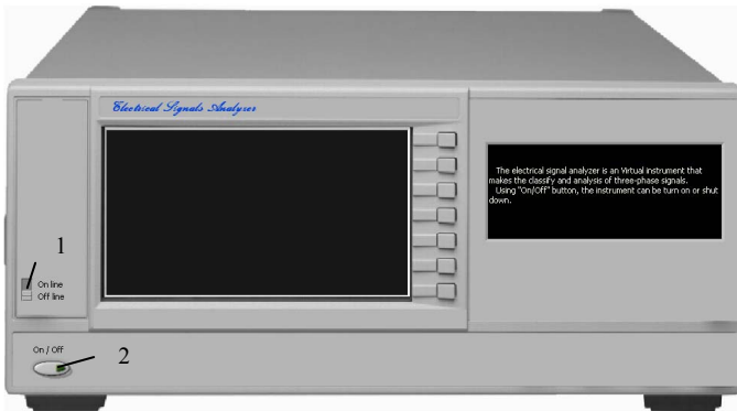
Fig. 1. Frontal panel of the electrical signal analyzer virtual instrument in shut down state. 1- On-line/Off-line button, 2- On/Off button
