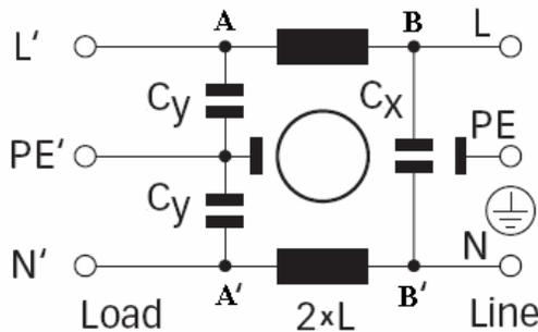
Fig. 2. Configuration of a power inlet filter.
