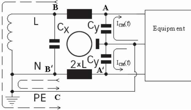
Fig. 4. Power inlet filters connected to the power distribution network. The upstream wiring impedance (loop impedance) is different from 50-Ω.
