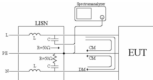
Fig. 1. Measurement of conducted emission using line impedance stabilizing network (LISN)
