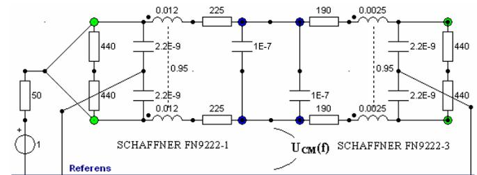
Fig. 5 The simulation of the common mode resonance is made by connecting two power inlet filters in parallel with the power distribution network and measuring the common mode voltage  $U_{CM}(f)$  between N-PE. In figure the PE is named reference.
