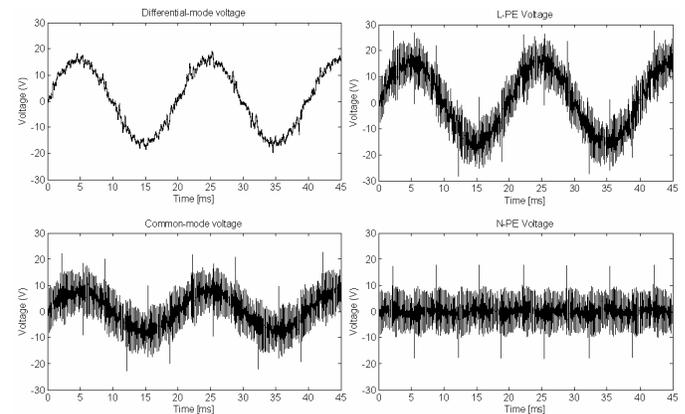
Fig. 8. The phase and neutral voltage in a server room measured with different references. The differential (L-N) voltage on the upper left, L-PE voltage on the upper right and the N-PE voltage lower right. Common mode voltage, to the lower left, is calculated from the measured L-N and L-PE voltage. The fundamental frequency voltage is attenuated 20 times in all cases.
