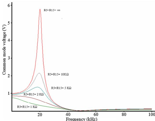
Fig. 6. Transfer function of the common-mode voltage over the power inlet filter, on the top in Table II, for different values of the loop impedance. The same loop impedance has been assumed in the line-earth and neutral-earth circuits.
