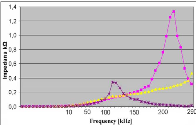
Fig. 7. Measured cable loop impedance between N-PE for three combinations of cables Yellow (triangles) 97 m N1XE-U 5G16 Magenta (squares) 213 m N1XE-U 5G10 Blue (stars) 50 m EKLK 3G1.5 + 213 m N1XE-U 5G10 + 97 m N1XE-U 5G16
