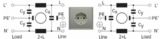
Fig. 3. Power inlet filters are connected in parallel with the power distribution network creating a sum of filter impedance different from 50- $\Omega$ .
