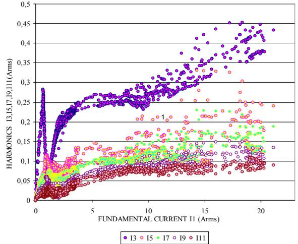
Fig. 2. Scatter diagram of Current Harmonics vs. Fundamental Current
