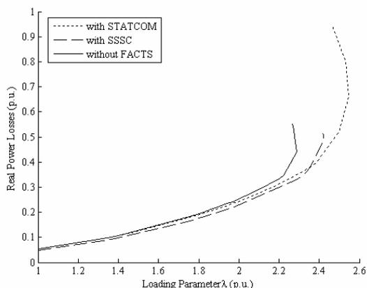
Fig.3. Impact of STATCOM and SSSC on real power losses
