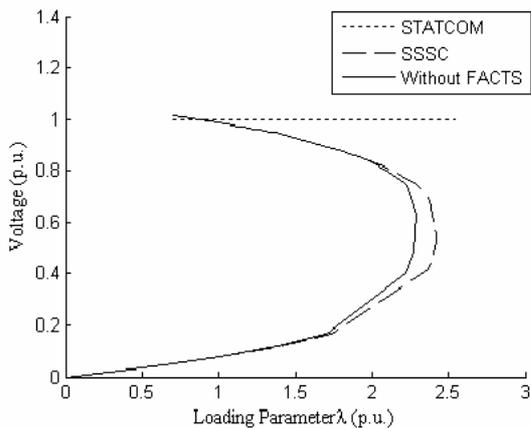
Fig.2. Impact of STATCOM and SSSC on static voltage stability margin.
