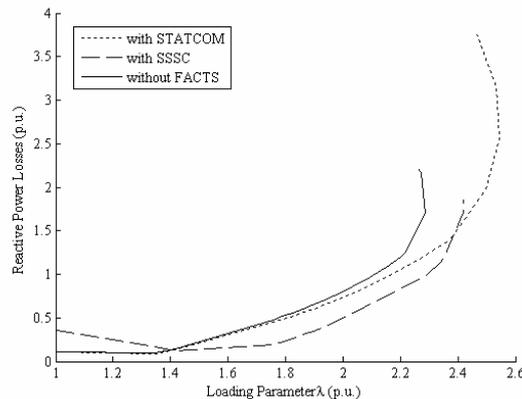
Fig.4. Impact of STATCOM and SSSC on reactive power losses
