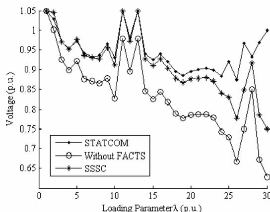
Fig.5. Impact of STATCOM and SSSC on voltage profile.
