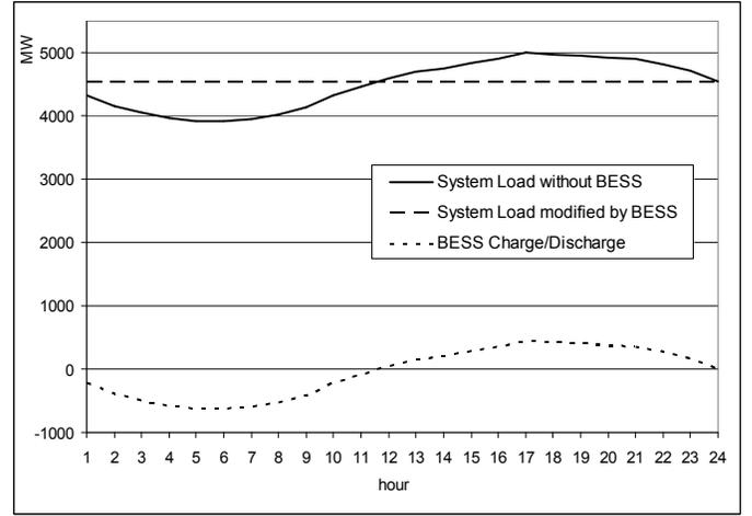
Fig. 2. System load leveling – Profile 2
