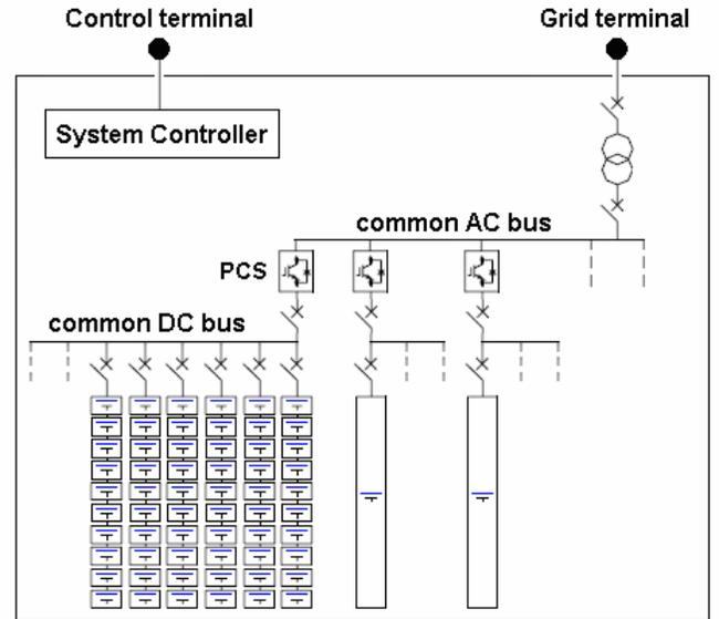
Fig. 5. Generic single-line diagram of one BESS block
