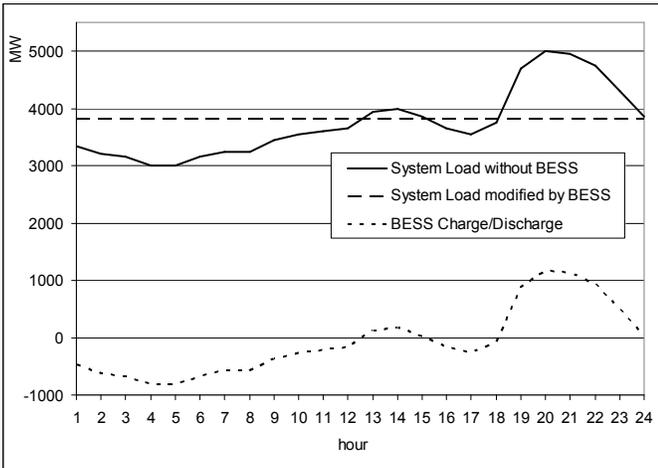
Fig. 1. System load leveling – Profile 1
