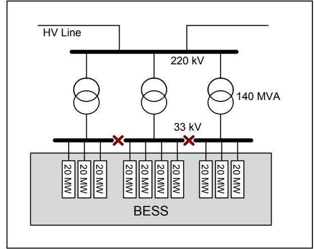
Fig. 10. Example of a 200 MW BESS in a S/S without loads
