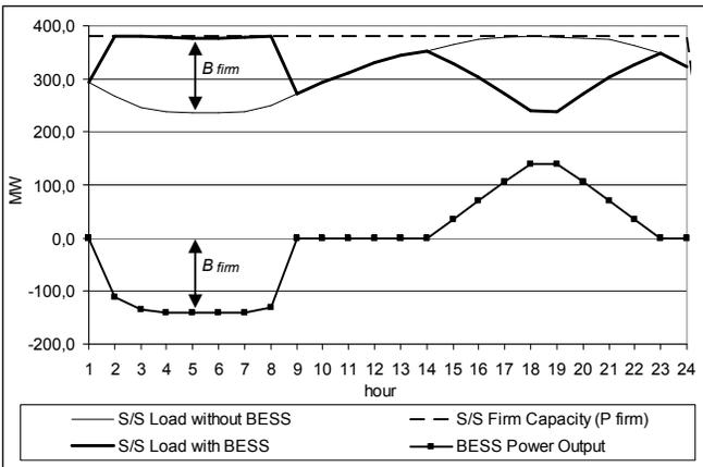
Fig. 6. Substation peak inversion 1 – BESS capacity =  $B_{firm}$
