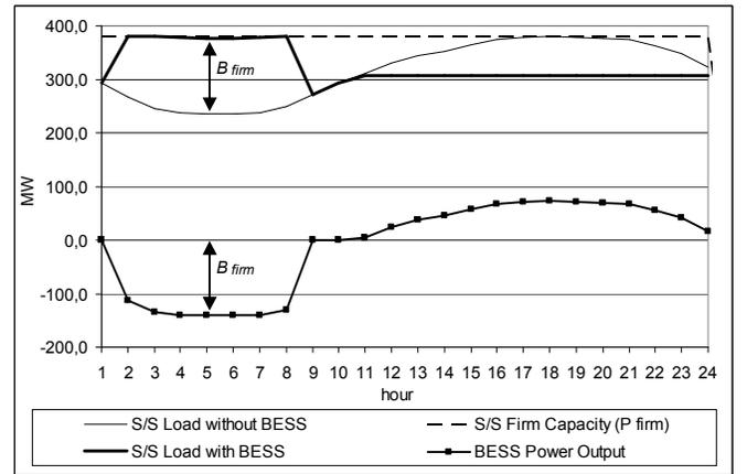
Fig. 7. Substation peak inversion 2 – BESS capacity =  $B_{firm}$
