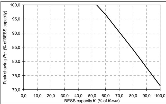
Fig. 4. Peak shaving (%) vs. BESS capacity – Profile 2
