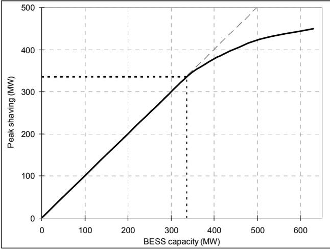
Fig. 3. Peak shaving (MW) vs. BESS capacity – Profile 2
